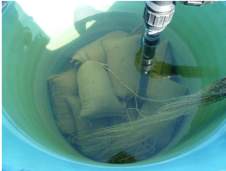
Figure 21. Bags containing the adsorption material inside the columns.
