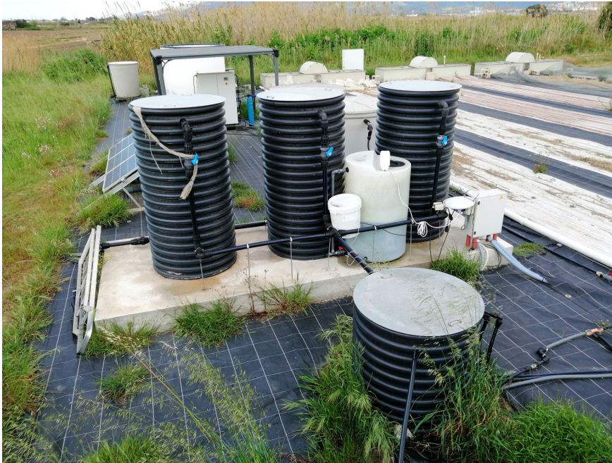
Figure 20. Adsorption columns for phosphorus recovery, with a tank and system for dosing extra nutrients to the influent water.
