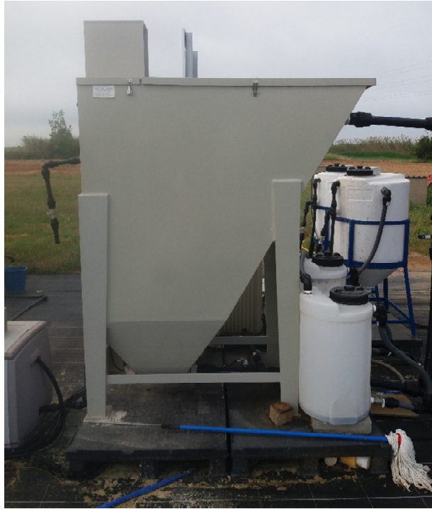
Figure 10. Side view of the lamella settling tank.
