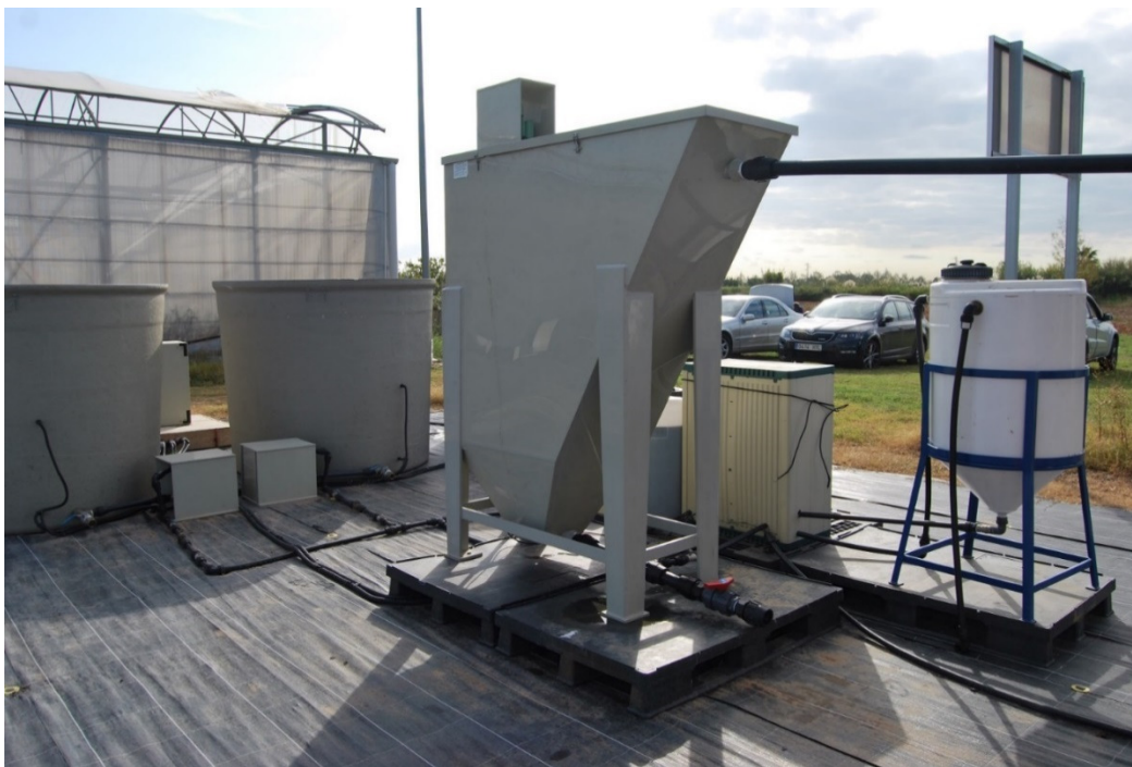
Figure 9. Lamella settling tank for biomass harvesting.
