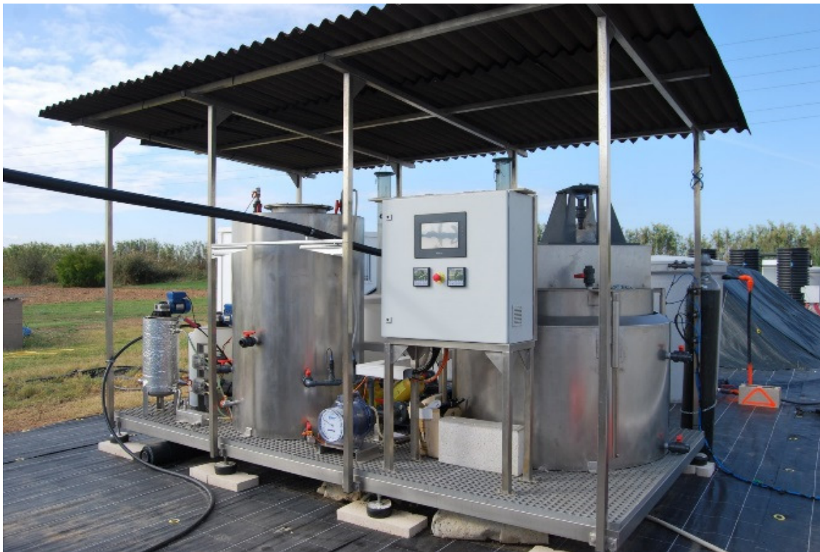
Figure 12. Anaerobic (co-)digestion plant: pretreatment (left), anaerobic digester (middle), and biogas storage tank (right).
