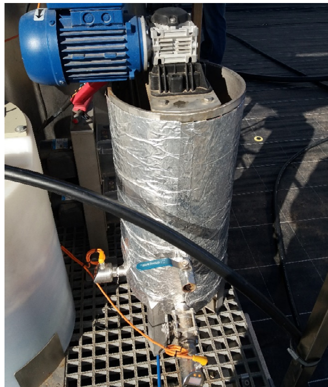
Figure 13. Tank for thermal pretreatment of microalgal biomass.
