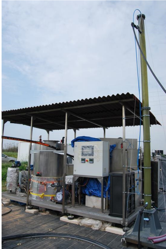
Figure 14. Absorption column for biogas upgrade to biomethane.
