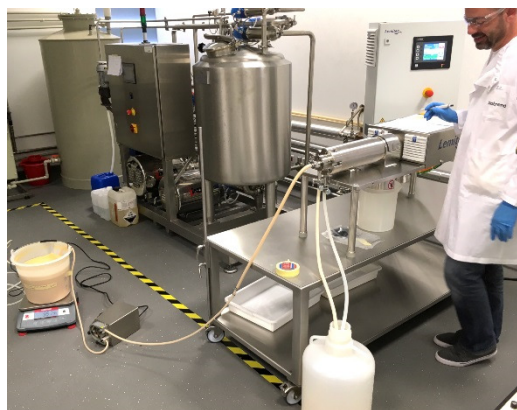
Figure 1.8: Biotrend's pilot plant manager testing the pilot scale centrifuge decanter with digested PHA-containing biomass.
