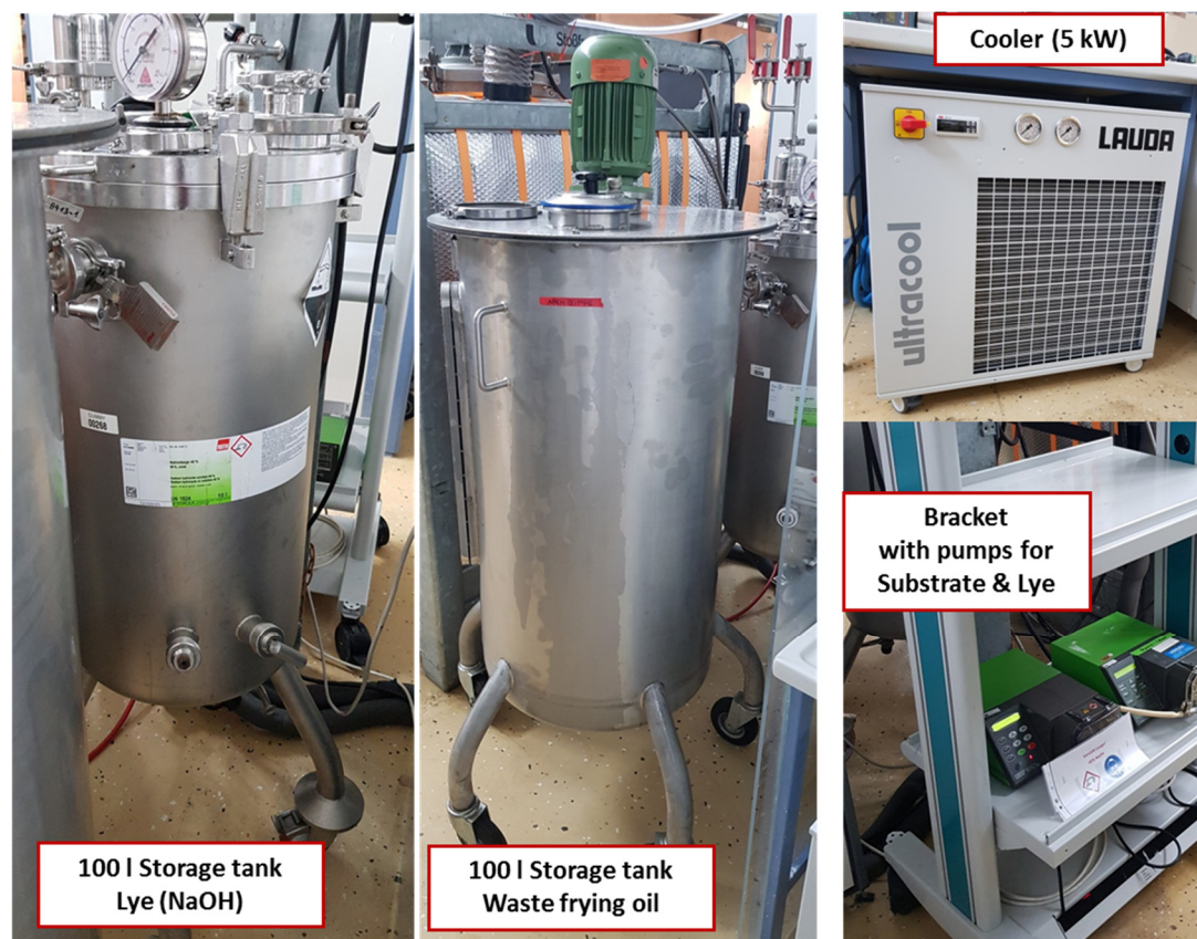
Figure 1.10 : Additional reactor equipment including storage tanks, pumps and a cooler.
