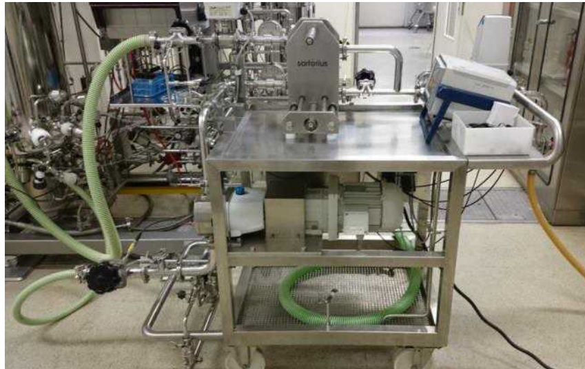
Figure 1.11 : Cross Flow Filtration (CFF) module for harvesting of yeast biomass by microfiltration.
