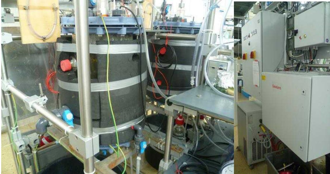
Figure 1.13 : 2 x 31 L Fermenters for one-stage biogas production (left) and control cabinet (right).
