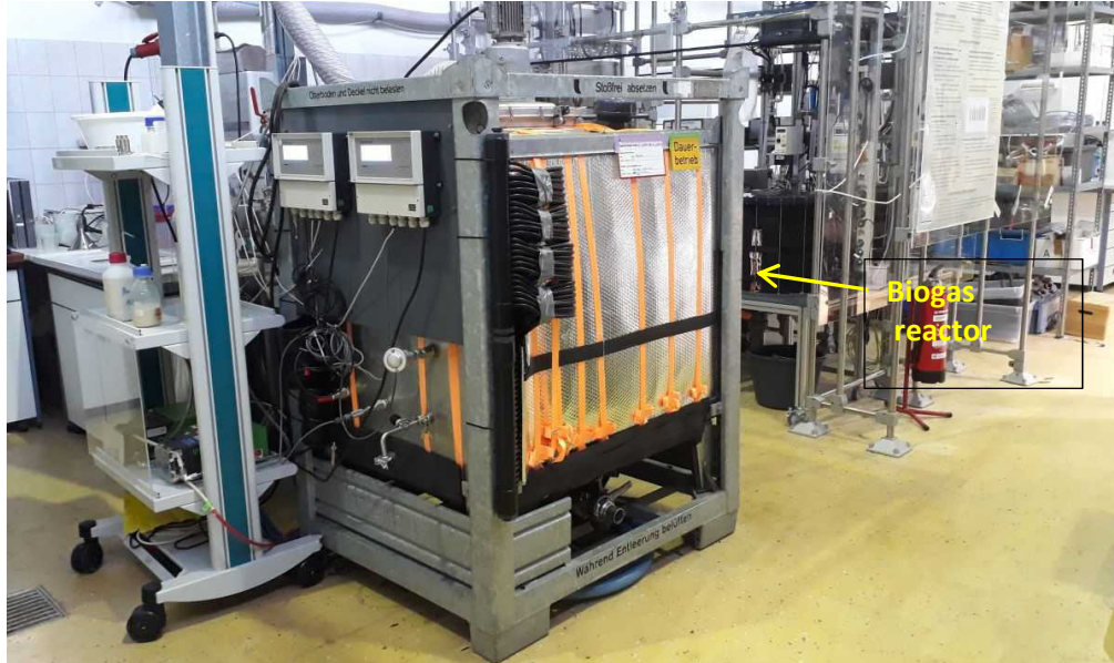
Figure 1.7 : Yeast bioreactor system based on IBC container (in the foreground) and biogas reactors (right in background).
