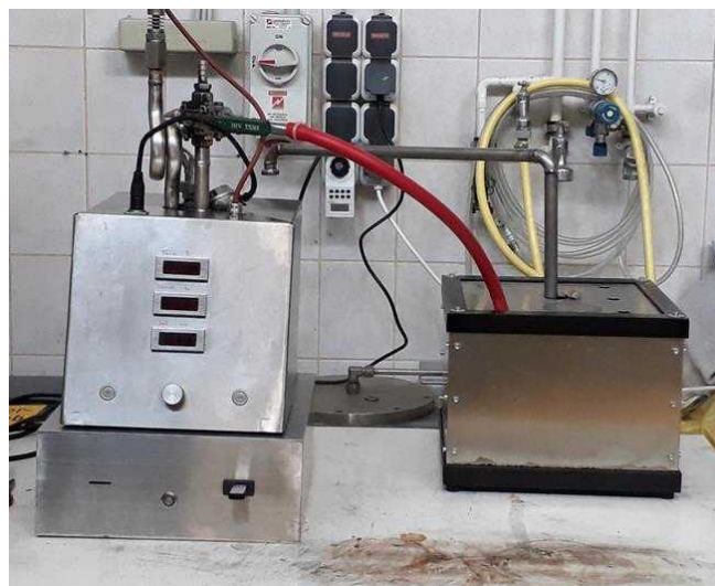
Figure 1.17 : 2 L laboratory scale HTC reactor system Autoclave Art. coal 2.0.
