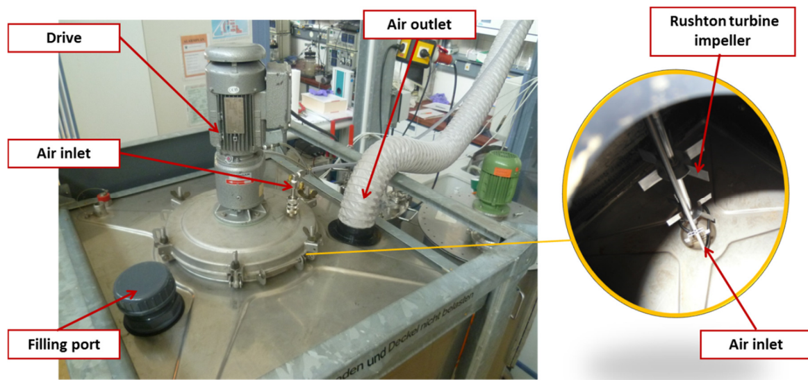
Figure 1.9 : Equipment on the top side of the yeast reactor.
