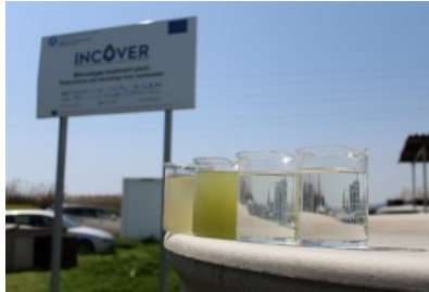
Successive steps of wastewater treatment with PBRs © UPC
